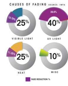
Window film does not completely eliminate interior fading, but it offers a reduction in the causes of fading. It reduces UV light, solar heat and visible light by blocking percentages of the causes. However, window film has no effect on items like dye fastness, age of fabrics and humidity, which is encompassed in the misc amount of 10% seen in the diagram.
